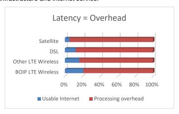
The above chart shows the performance impact of network latency on 100 mbps of internet bandwidth with no account for packet loss. The average latency for BOIP competitors is published in the 2018 FCC report on broadband. BOIP's latency is an average of our deployed customer's latency numbers.
